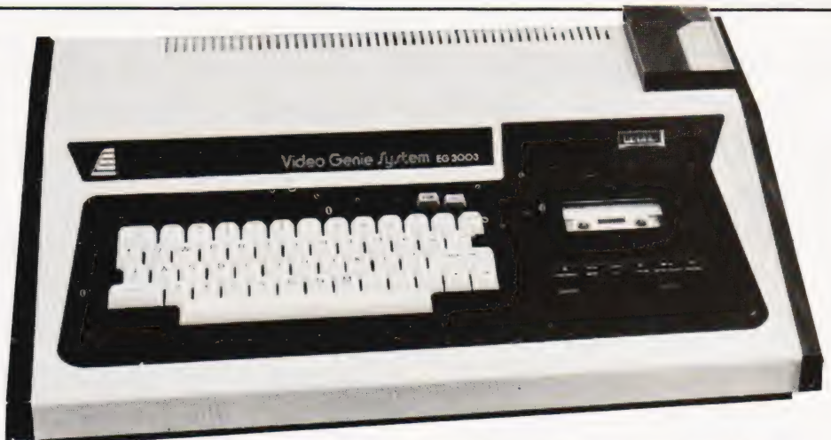
The Genie keyboard unit. The PAGE and F1 buttons referred to in the text are located top right.
